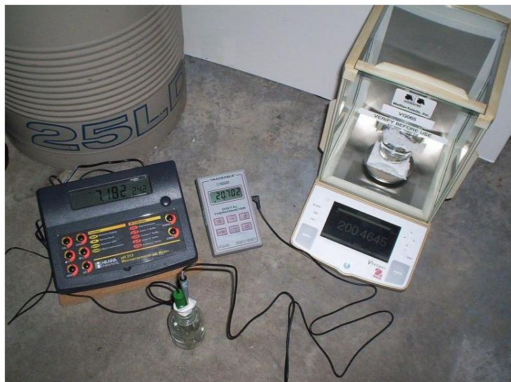
Figure1. Illustration of the key experimental setup. Several variations of this setup were also used in the actual experiments as described in the text. For example, in one variation, the manipulation was heating the water in the 3 rd reservoir to boiling point and then cooling it down. In a second variation, the gravity measurement was eliminated and the manipulations were first adding 5ml concentrated HCl (30%) to the third reservoir, then adding 20g NaOH to the same and third heating the same to boiling point. In a third variation, the Dewar was located more than 500 feet away from the site of measurement. In fourth variation, the gravity and pH measurements were eliminated and the temperature measurements were carried out more than 50 miles away from the location of the Dewar.
